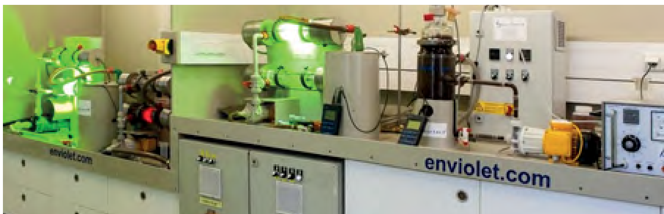
Laboratory scaled Enviolet® UV-plants (UV-reactors with different types of light sources)
