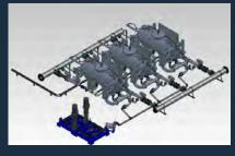
The main treatment stage consists of three AMF<sup>2</sup> 370K microfiber filters at 2 micron filtration degree.
