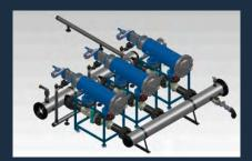
The first stage of filtration, designed to remove large suspended solids from the raw water, consists of a battery of SAF 6000 series automatic screen filters with 80 micron filtration degree and stainless steel screens.
