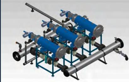
**1** The first stage of filtration, designed to remove large suspended solids from the raw water, consists of a battery of SAF 6000 series automatic screen filters with 80 micron filtration degree and stainless steel screens.
