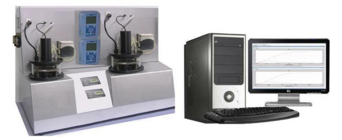
Traditional studies of this nature could only focus on a very narrow area, such as nitrification inhibition in one specific set of conditions. The BM-Advance2 allows for the study of multiple issues across multiple operating conditions – all in a highly controlled and verifiable environment – bringing Pilot Plant Studies to a new level.
